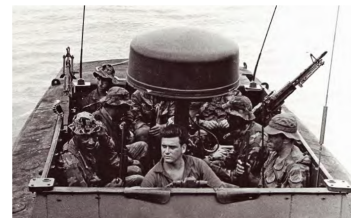
The LSB was a squad-sized boat with water-jet propulsion and an exceedingly small draft that could get into very shallow-water regions.
