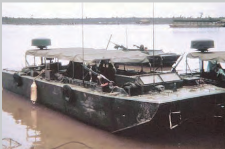
The MSSC was a platoon-sized boat with a shallow draft and propelled by water jets. It had a top speed of over 35 knots.
